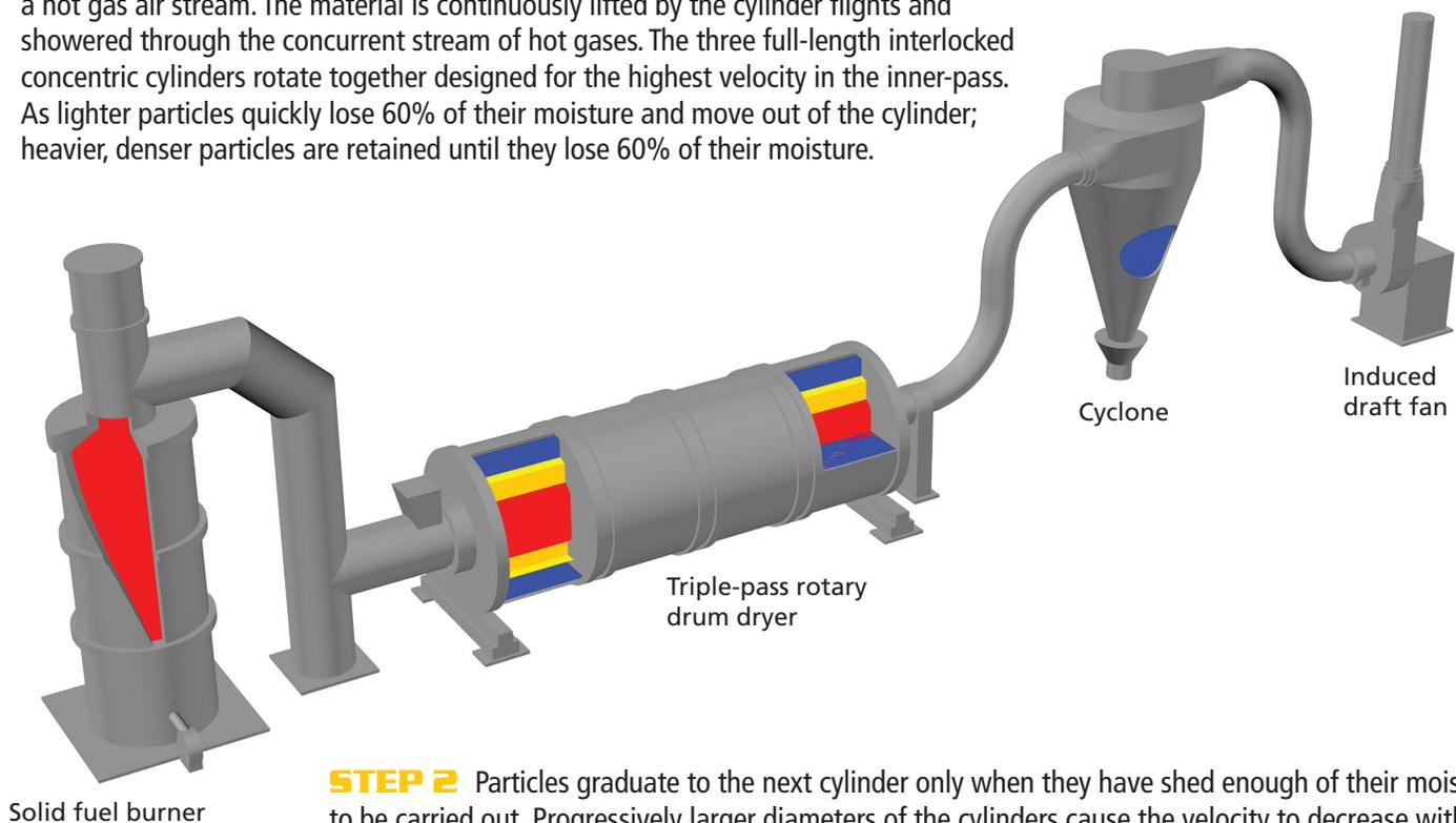
**STEP 2** Particles graduate to the next cylinder only when they have shed enough of their moisture to be carried out. Progressively larger diameters of the cylinders cause the velocity to decrease with each subsequent pass. In this section, the partially evaporated particles are handled more gently, again only graduating to the next pass when they have shed the proper amount of moisture.
